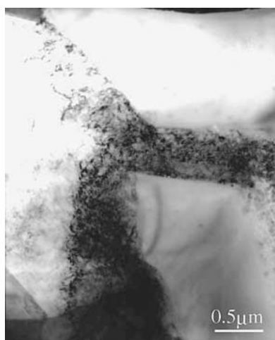
Figure 9 High-density dislocations in the composite.
